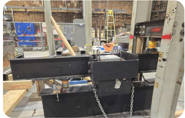
Test set up for modified bond-wrench
